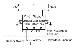
Fig. 2. Connection Diagram: Model SBG41705
